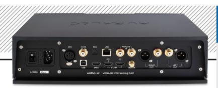
ABOVE: Digital inputs on AES, coaxial and optical (192kHz/24-bit and DSD64 over DoP) are joined by wired LAN, USB-B and Auralic Lightning Link ports (384kHz/32-bit and DSD512) plus an external clock input. Line inputs (on RCAs) sit alongside fixed/ variable preamp outputs on XLRs (balanced) and RCAs
