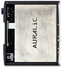
ABOVE: Hidden within the alloy chassis, and screening the circuitry within, is a branded nickel-plated copper enclosure
