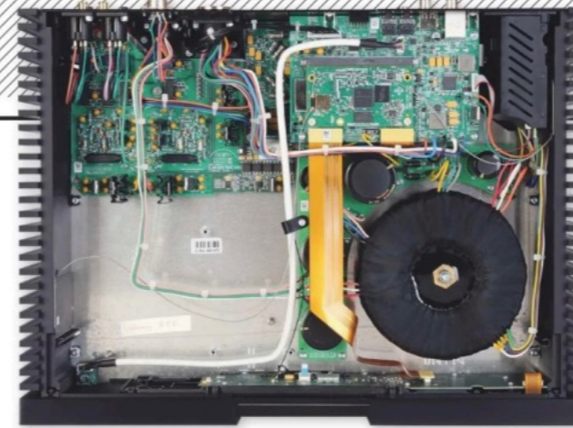
ABOVE: The NSS 333's large toroidal transformer [bottom right] feeds 4x PSUs for the NP800 streaming card [top right], ARM CPU [top right, centre PCB], DAC and SHARC DSP [top right, lower PCB] and Class A preamp stage [top left]
