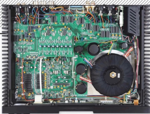
ABOVE: The NAC 332’s toroidal transformer [bottom right] feeds 4x PSUs supporting the Class A input buffers [top left], balanced to single-ended preamp [centre], R-2R reed relay volume circuit [bottom left] and ARM microprocessor [bottom right]
